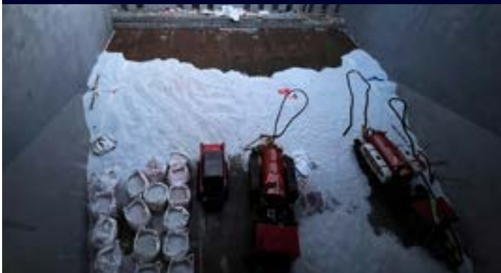
Product Salvage Operation Using Vacuum System
