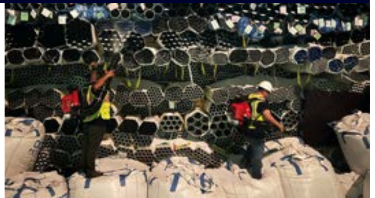
Cleaning Contaminated Steel Pipe Product
